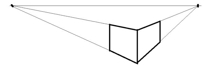
Step 4: draw two auxiliary lines to close the top face and redraw the edges with definitive lines.
