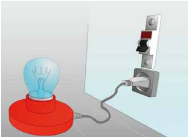
Automatic control switches or circuit breakers
