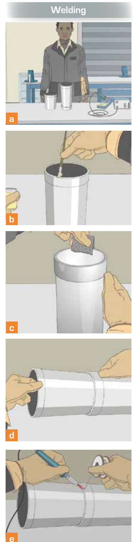
b) The flux is applied c) the joint area is filed d) the pieces are fitted together e) the joint area is heated and the filler metal is applied.
